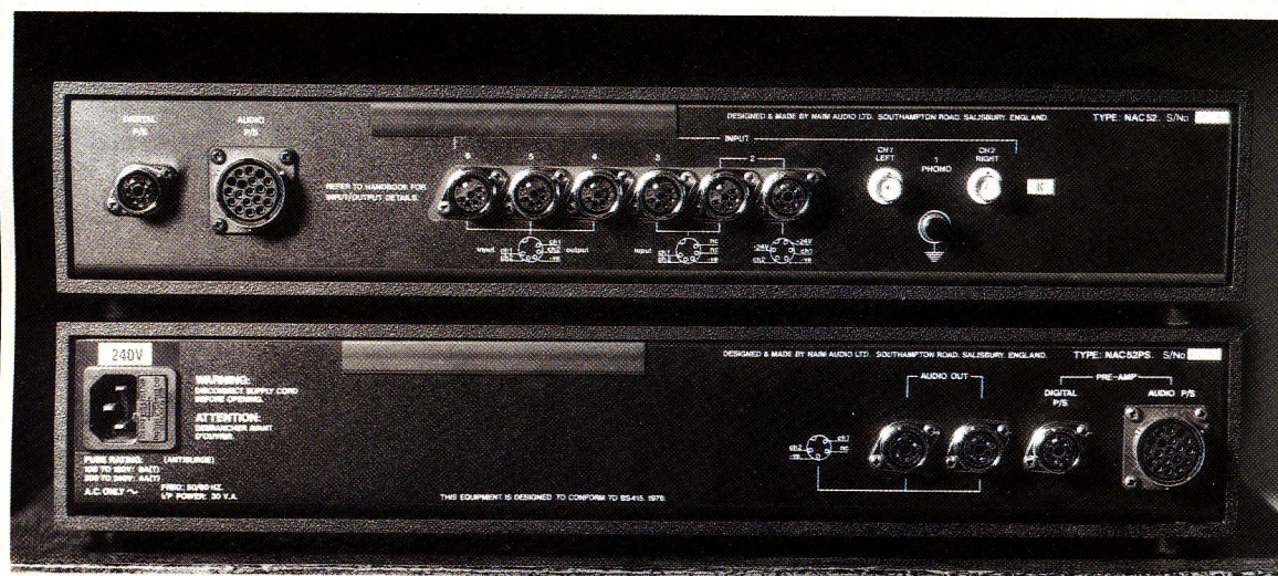
Rear view of the NAC52 (top)/ NAC52PS (below) combination shows DIN sockets in abundance, plus large 16-pin socketry for the hawser-like cable that connects the two together. Phono input, meanwhile, uses the BNC sockets preferred by Naim
