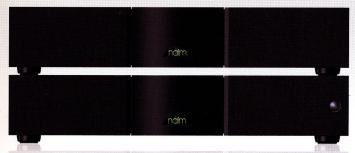
Like our flagship amplifier, NAP 500, the NAP 300 is a stereo twochassis amplifier, one case containing the audio amplifier and the second housing the regulated power supply. It also uses the same 007 transistors that were custom-designed for the NAP 500. The NAP 300 has a huge 500VA transient ability, and a power output per channel of 90W into 8 ohms. The NAP 300 delivers awesome power without sacrificing any speed or agility.
